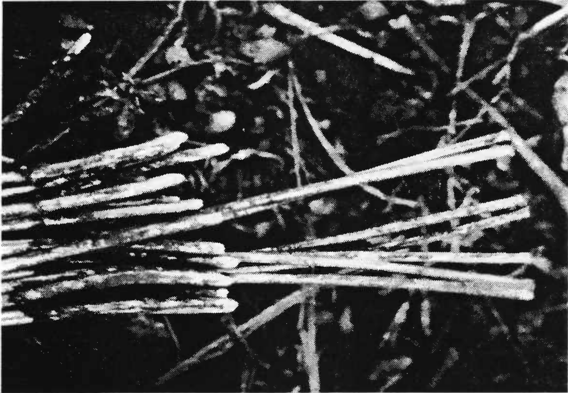
Fig. 1-5 (a) : Conductor tension failure
